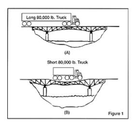
In Figure 1(A), the stress on bridge members as the longer truck rolls across is much less than that caused by the short vehicle in Figure 1(B), even though both trucks have the same total weight and individual axle weights. The weight of the longer vehicle is spread out, while the shorter vehicle has all of the weight concentrated on a small area.
