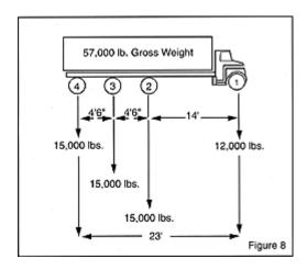
The truck in Figure 8 satisfies the single axle weight limit (12,000 lbs. is less than 20,000 lbs.), the tandem axle limit (30,000 lbs. is less than 34,000 lbs.) and gross weight limit (57,000 lbs. is less than 80,000 lbs.). With these restrictions satisfied, a check will be made for Bridge Formula requirements, axles 1 through 4.
