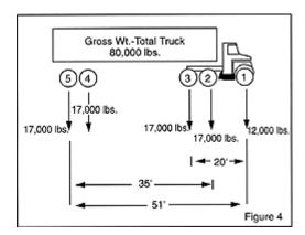
Before checking a vehicle for compliance with the Bridge Formula, its single-axle, tandem-axle, and gross weight should be checked. Here the single axle (number 1) does not exceed 20,000 lbs., tandems 2-3 and 4-5 do not exceed 34,000 lbs. each, and the gross weight does not exceed 80,000 lbs. These preliminary requirements are thus satisfied. The first Bridge Formula combination is checked as follows:
